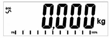
The scale has an automatic re-zeroing function to account for minor drifting
