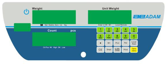
The scales have three display windows- Weight, Unit Weight and Count.
