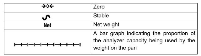
Note: Some symbols shown on the display are not used in the analyzers. During the moisture test the main display will show the percent moisture. It can be switched to other values using the **[Dspl/**] key. For example current mass.
